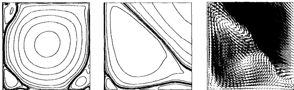
FIG. 11. Solution after 150 iterations for Re = 15,000 with the 256 \times 256 grid.
